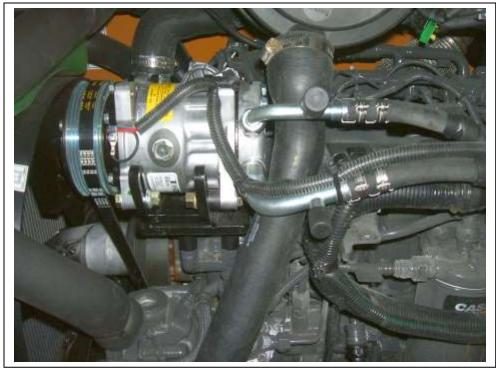
New engine configuration with air intake hose. Install NAR sleeving over hose to protect from rubbing on the fittings.
