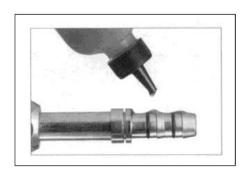
Step 4. Insert the nipple into the hose. To ensure that the nipple is fully inserted, check the gap between the cut end of the hose and the shoulder on the nipple. Care should be taken to avoid kinking or other damage to the hose during nipple insertion. NOTE: Be sure to wipe excess oil from the nipple and hose.
